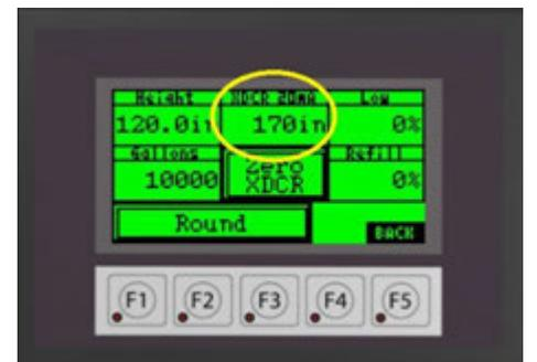
Once the tank shape, height and volume have been set, the level transducer for the tank must be calibrated (zeroed). To do so, remove the probe from the tank or hold it above the fluid level and press and release the **"Zero XDCR"** button several times to verify the measurement is accurate. When finished, install/return the probe to the tank. (See **Zero Transducer**)
