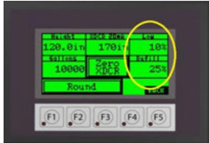
Enter the level in percent the system should generate a Refill Reminder Warning. Should a tank reach this level, a warning will be generated to inform the site personnel that a fuel delivery should be scheduled. Entering "0" disables this feature. (See *Low Fuel Setpoint/Refill Warning*)
