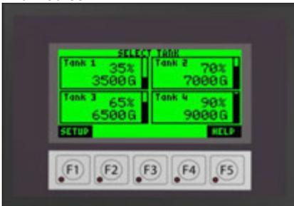
Repeat the process for each tank in the system. The main screen will now show the active tank information. The current percent and gallons/liters will be displayed for each tank. (See *Main Screen*)
