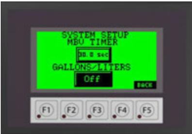
If Motorized Ball Valves (MBV) are installed, you may enter the delay time in seconds for the valve fail timer. You may also select to display the tank level in either GALLONS or LITERS. Tank level in percent will always be displayed regardless if gallons or liters is selected. (See *System Setup*)
