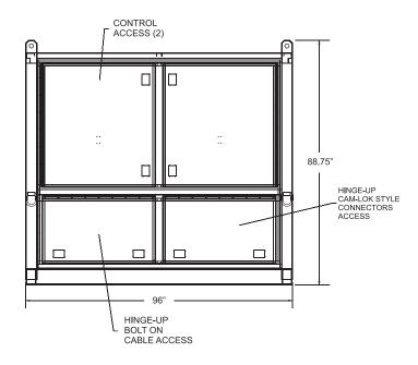
The Load Bank is a completely self-contained, freestanding unit which includes all inductive load elements, load control devices, load element branch circuit fuse protection, main load bus and terminals, cooling system, control power supply, unit controller and malfunction detection system.
