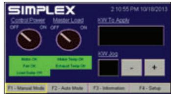
**Figure 23 HMI - Manual Mode**
