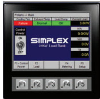
Figure 37 Cooling Fan Failure
