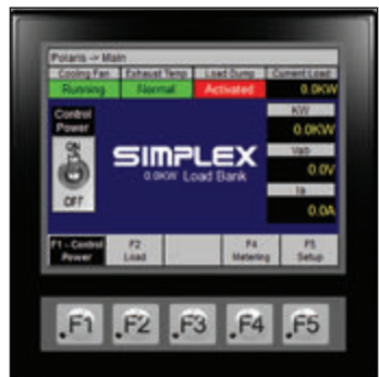
Figure 39 Load Dump Activated
