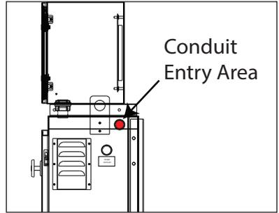
To bring cabling into the SmartFilter, pull a hole into the cabinet in the Conduit Entry Area (see **Figure 2**) and install a 3R-rated conduit connector for access.
